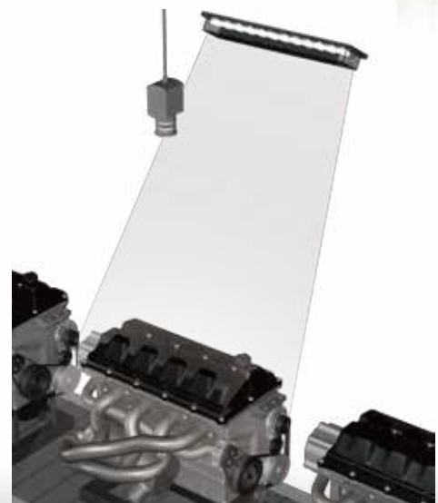
Inspection for the existence of engine parts
