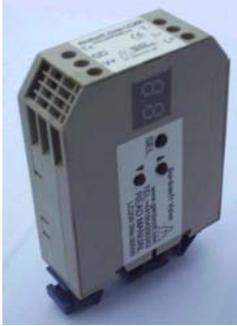
The LC200 lighting controller provides repeatable intensity control of LED lighting for machine vision applications. It includes the power regulation, timing and triggering functions required for machine vision systems. Two modes of operation are provided:
