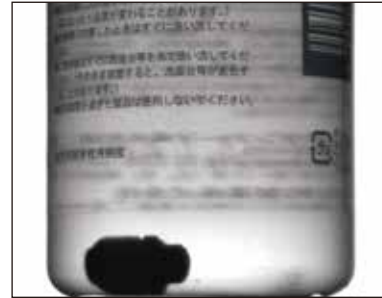
Imaging with infrared light penetrates the liquid and captures the foreign materials.
