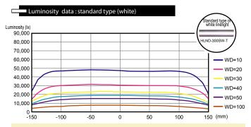
Using a high-diffusivity diffuser achieves compatibility between high light intensity and even illumination, thus executing power for imaging in bright fields with specular and transmitted light in use.
