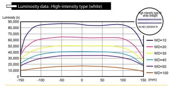
Using a high-transmittance diffuser ensures very high light intensity and even illumination with no extreme fluctuations in the intensity, thus executing power for imaging in dark fields with scattered light in use.
