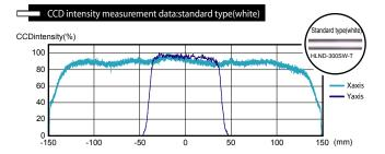
For the standard type of white linelights, light illumination within the effective illumination area of 200 mm in width is able to produce a uniform light with no extreme fluctuations.
