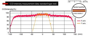
For the standard type of red linelights, light illumination within the effective illumination area of 200 mm in width is able to a uniform light with minimized fluctuations.
