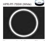
You can check the condition of an O-ring surface by brightly and evenly illuminating it.
