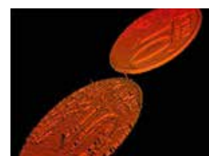
ELL (up) VS LASER (down): no speckle = more accurate
