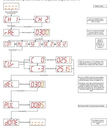
Extended Set Up can be used to set pulsed output as follows.
