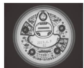
At LWD of 200 mm, the bumps and pull tab are emphasized.
