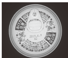
At LWD of 10 mm, the whole surface of the workpiece is illuminated uniformly. The bumps are eliminated from the image.
