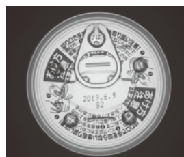
At LWD of 100 mm, the bumps and pull tab are captured.
