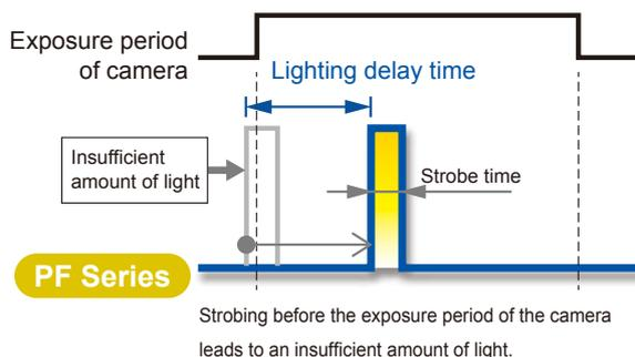
Delaying the timing of the flash enables strobing **within the exposure period** of the camera.
