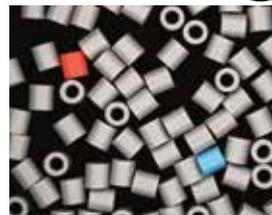
You can check for resins of different colors by combining the light with a color camera.
