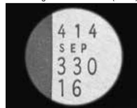
Evenly illuminate the entire surface of a capacitor by combining dome type and coaxial type lights.
