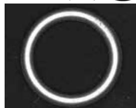
You can check the condition of an O-ring surface by brightly and evenly illuminating it.
