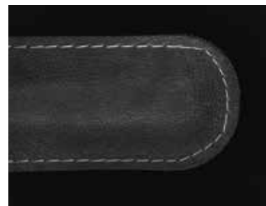
Infrared light penetrates the dye to highlight the threads and captures the stitching.
