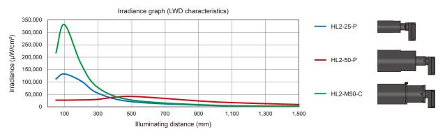
Measurement with HLV3-22SW-4S (white) mounted on the lens. Measured values using our measurement conditions. Results for individual products may vary
