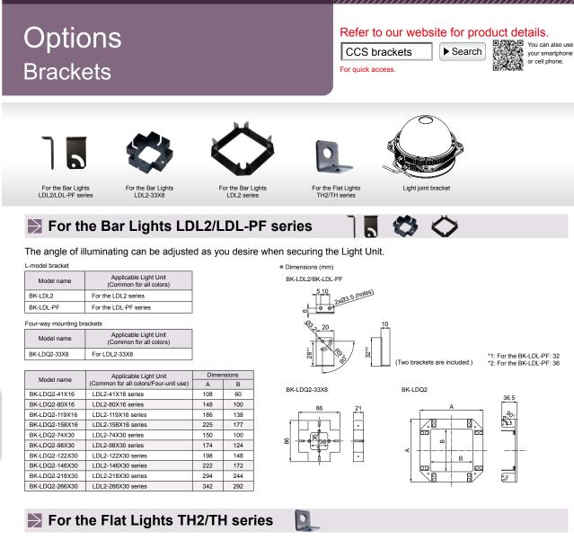
This is a dedicated bracket for securing the TH2/TH Series Light Units. You can secure the Light Units at four points.
