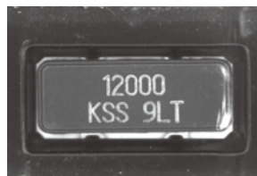
Surface reflection is reduced and an image of the text can be made.
