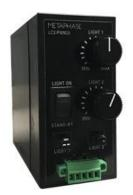
The LC2-PWM20 is a dual channel, pulsewidth modulated LED intensity controller. It outputs 12V PWM from 0-100% at 100kHz to drive LED loads with series limiting resistors. The maximum output is 20W per channel and 30W combined for two channels. Power is limited by the 24V power supply.
