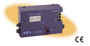
By connecting the STU-3000 to CCS's PD2 Series digital control units, a constant lighting unit can be used as a strobe light. The one-shot circuit in the adaptor is activated by external trigger signals, the power ON/OFF supply is controlled at a defined pulse width, and an LED light is flashed as a strobe light. The strobe flash time can be set between 0.01 and 99.99msec. by means of the four-digit digital switch.
