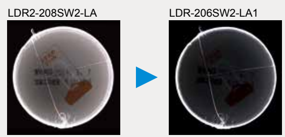
The seal and engraved text affect the image, and the shrink seal cannot be sufficiently detected. Only the shrink seal clearly stands out.
