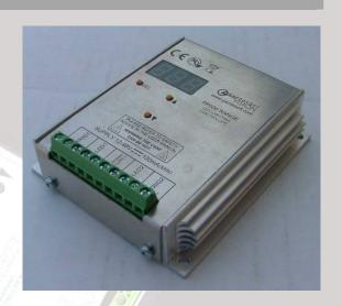
The PP500/PP520 Range has options for normal or fast pulsing and with or without Ethernet interface.
