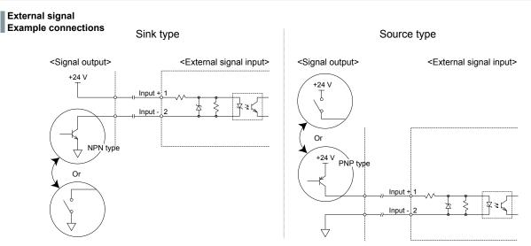
Becomes HIGH when 24 V is applied to input+ and 0 V is applied to input-. Apply a current using the open-collector circuit, high-speed photocoupler, semiconductor relay, and so on. (We recommend 10 mA or less.) The pulse width must be 10 µs or more (Applied voltage 24 V±10%).
