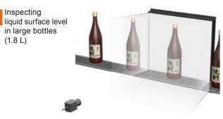
Workpiece image Large bottles (1.8 L) Height: 400 mm
