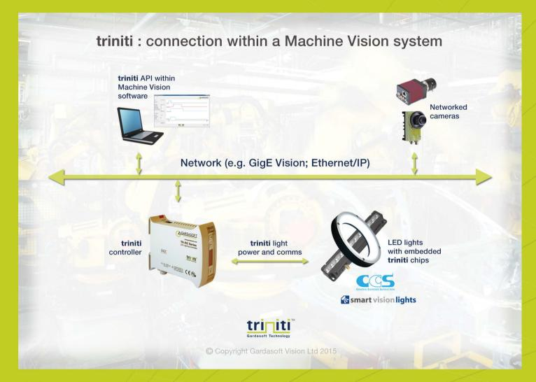
triniti also exploits standard Machine Vision networking and communication architectures such as GigE Vision and GenlCam, in order to ensure that the resulting solutions are fully integrated (as illustrated above, and as follows):
