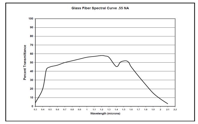
NOTE: Spectrum shown is for the fiber optic only, and is not representative of output spectrum when paired with a light source and lensing.
