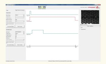
The TR-HT Series can also be configured using simple string commands sent from within their application program using RS232, TCP/IP or UDP, and the Triniti SDK (which is a free download from the Gardasoft website). The configuration is stored in non-volatile memory providing turnkey operation.
