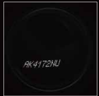
Example of imaging with UV-LED lighting
