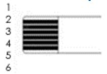
\*cable side pin designation matches Molex 52746-0671 bottom side contacts connector
